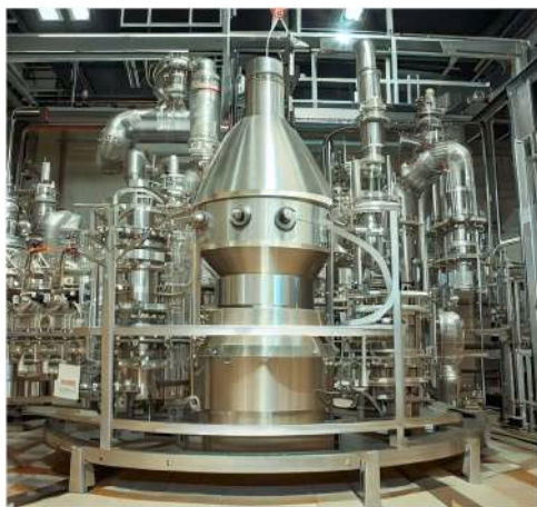
Fig. 4. Rotating cone reactor, Shell OMEGA process with cyclic distillation for pharmaceuticals purposes [69].
