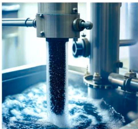
Fig. 1. Adsorptive removal of Ni(II) ions from a stream of subcritical water using an activated carbon fixed column. Reske et al. [26].
